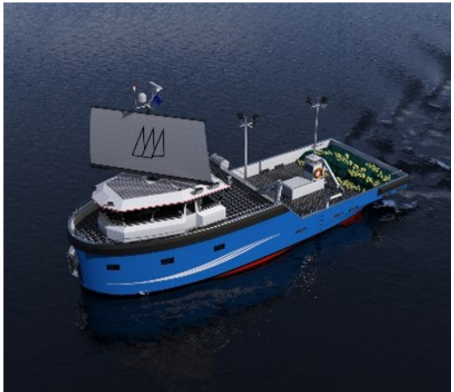
Figure 3: Project “Sailfish” wind-assisted fishing vessel (Source: MPENG, Barcelona)
