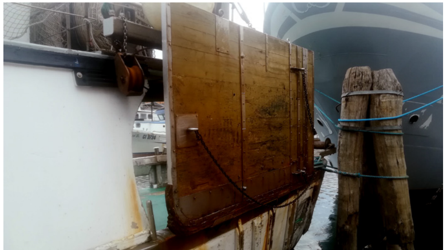
Figure 7: Otter boards with wood panels in use in the Chioggia otter trawl fleet, Italy (Source: DG MARE, July 2022, Sept. 2022)
